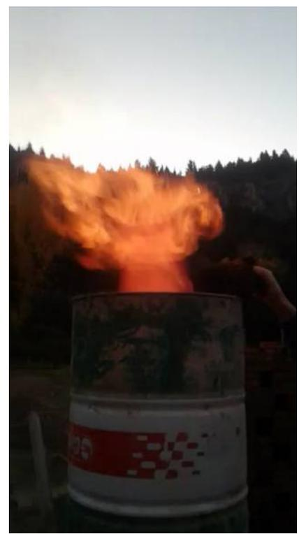
*Picture 16: We realize we can contain these flames adding more height of heat riser*
