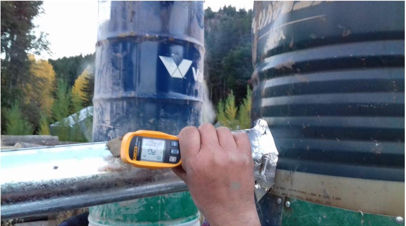
*Picture 23: 19:20 pm (40 minutes of burn). Point 1. Reading 121,2 °C*
